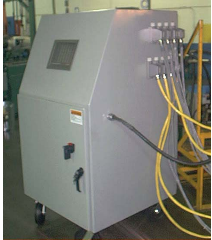
Panel with prefabricated plug-in cables for heaters and thermocouples
