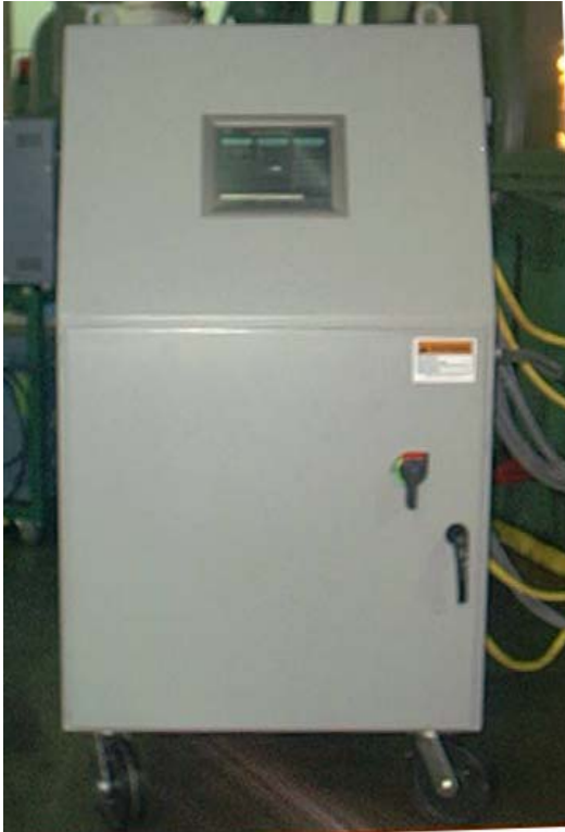
Front view of cabinet. Touchscreen operator station.
