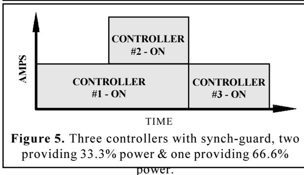
**Figure 5.** Three controllers with sync-guard, two providing 33.3% power & one providing 66.6% power.
