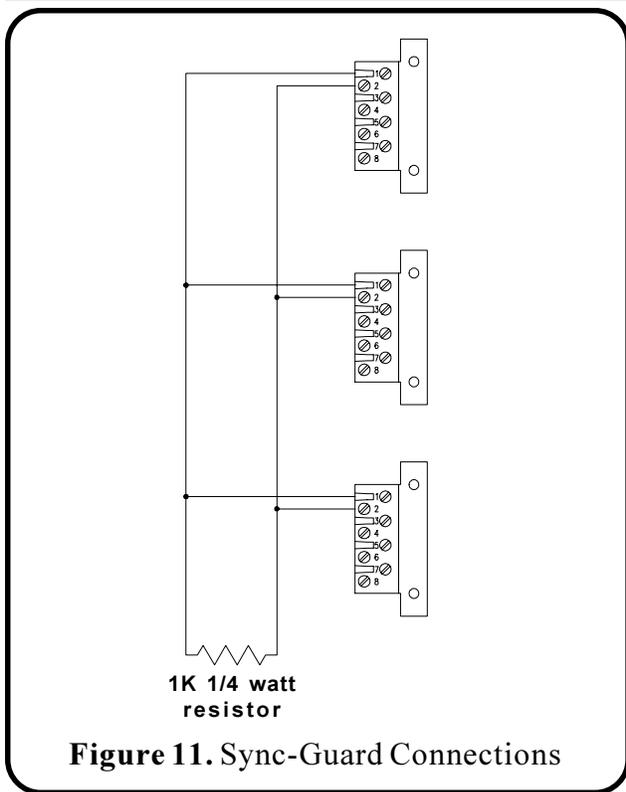
Figure 11. Sync-Guard Connections
