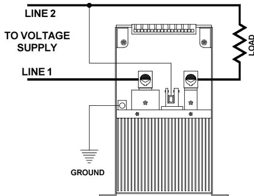
Figure 8. Power connections.
