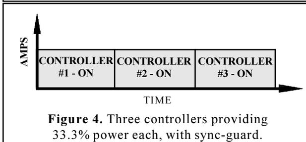
**Figure 4.** Three controllers providing 33.3% power each, with sync-guard.
