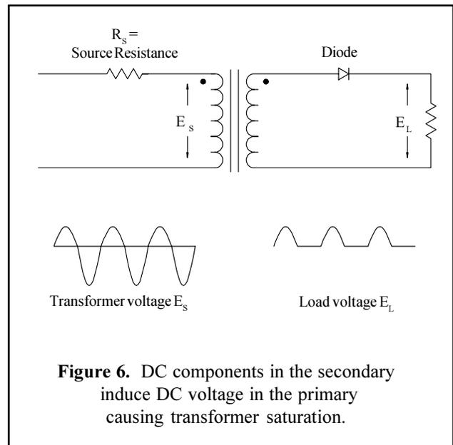
**Figure 6.** DC components in the secondary induce DC voltage in the primary causing transformer saturation.
