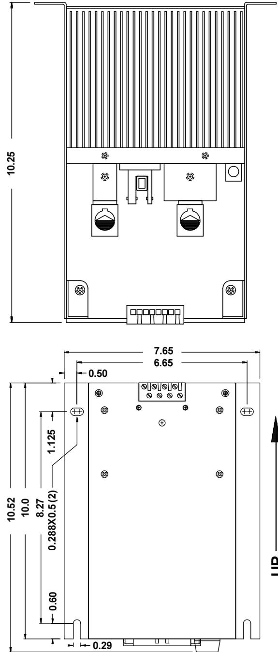
**Figure 7.** Installation drawing for 50 to 160 Amp models.
