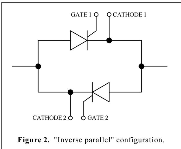
Figure 2. "Inverse parallel" configuration.
