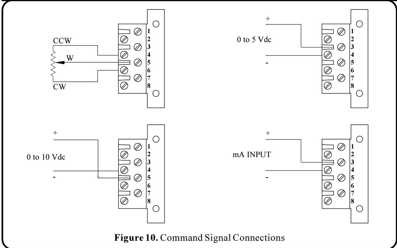
Figure 10. Command Signal Connections
