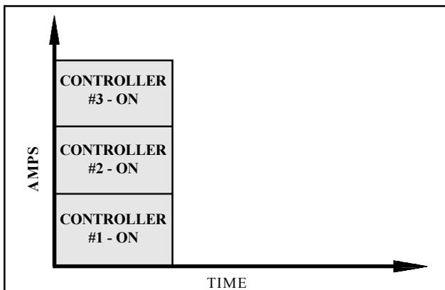
**Figure 3.** Three controllers providing 33.3% power operating synchronously.
