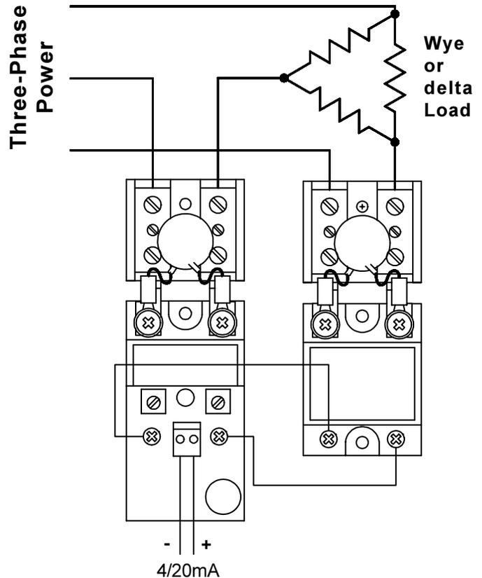
The model 3020 control circuit is powered by the current loop command signal. It does not require a transformer.
